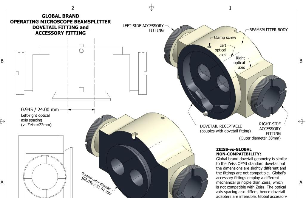
axis spacing also differs, hence dovetail adapters are infeasible. Global accessory ports can be mechanically adapted to accept Zeiss attachments, and vice versa, subject to optical stop limitations on length.
