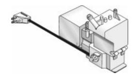
As the water level rises to contact the high water cut-in probe in the reservoir, a signal is sent to the electronic control board. The control board performs a low voltage comparison by water contact between the high water cut-in and common probes. If water is contacting both probes the pump motor turns on and the pump runs.
