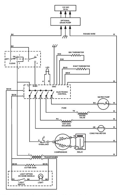
Wiring Diagram shows unit in Ice Making Mode
