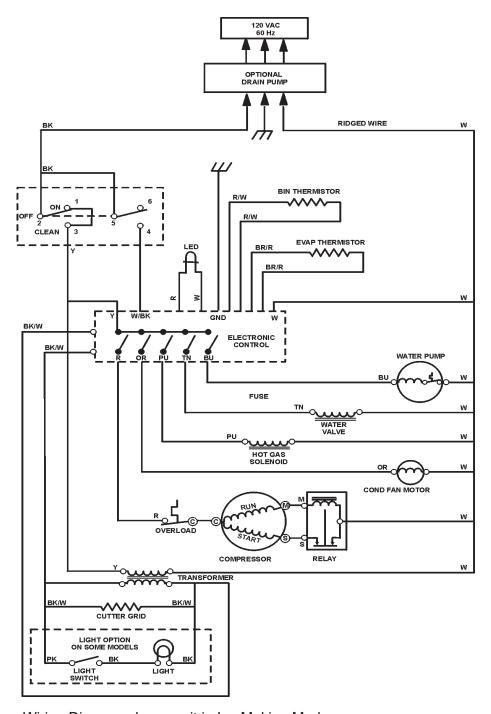
Wiring Diagram shows unit in Ice Making Mode.
